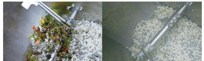
Raw garbage disposal unit installed (left: immediately after garbage added; right: 24 hours later)
